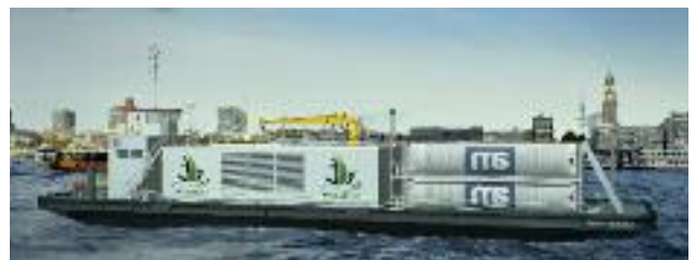
MS power barge: powered by LNG
